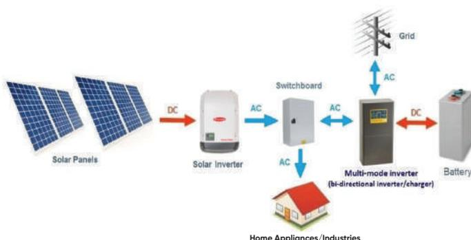
(Solar - Inverter Connection Diagram)
